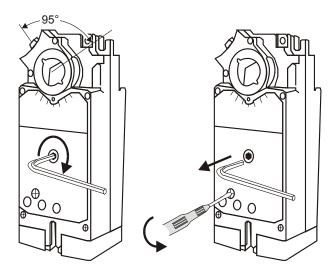
Fig. 3. Manual positioning
