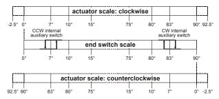
Fig. 4. Internal end switch triggering points
