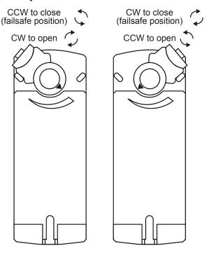
Fig. 2. Mounting orientation
