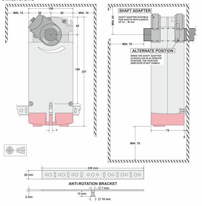
Fig. 8. Dimensions (in mm)
