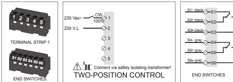
**NOTE:** Internal end switches S1 and S4 must be connected to the same power source.
