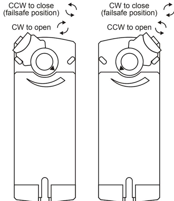
Fig. 2. Mounting orientation
