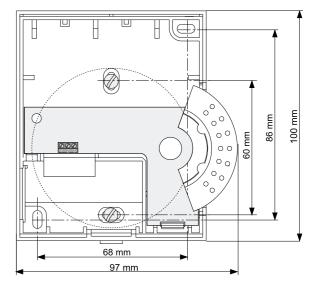
Figure 2: Installation onto flush distribution box
