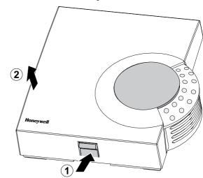
Figure 1: Removing housing cover
