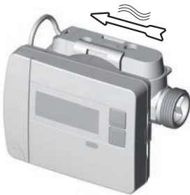
Tilted horizontal installation
