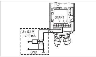
Fig. 2 Remote control digital
