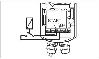
Fig. 3 Differential pressure switch
