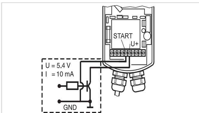
Fig. 2 Remote control digital
