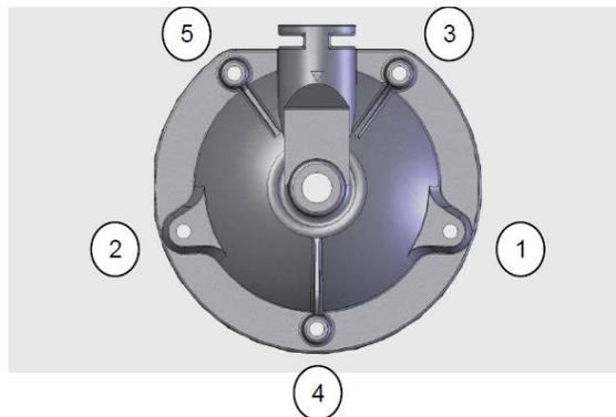
3.18. Unscrew and remove Injector Housing Cap by turning the cap counter-clockwise by hand
