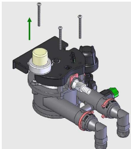
3.10. Lift off the motor plate taking care to ensure that the drive gear sensor is not damaged.
