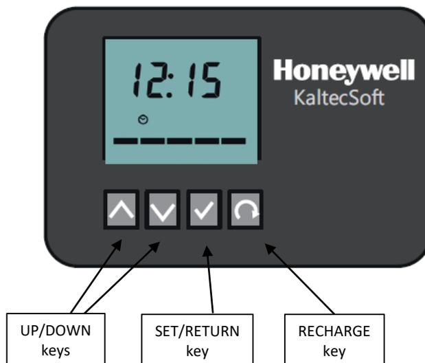
Pressing the SET / RETURN key once the time is set moves the display to set hardness mode
