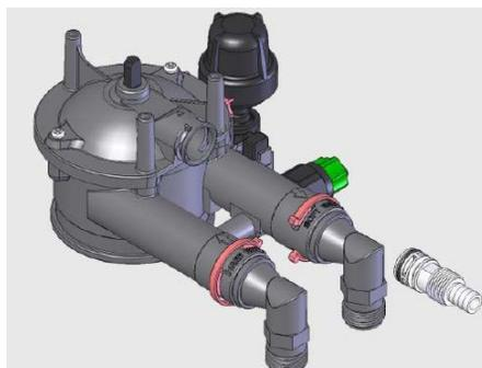
3.13. Remove the 2 remaining top cover retaining screws from the top cover
