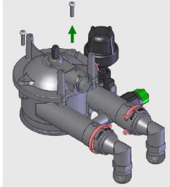
3.14. Lift off the valve top cover. Normally the valve rotor assembly and associated seals and springs will lift out with the top cover
