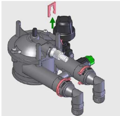
3.12. Pull the drain hose adaptor from the main valve top cover port. Check the condition of the O-ring seal on the adaptor. This seal is not a wear seal and should not require replacing as standard during a routine service but if any damage or degradation is found replace the O-ring as a precaution. Ensure that whenever a seal or O-ring is replaced it is greased with a suitable silicone based lubricant.
