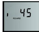
Once fill position has been reached a countdown timer will show the time remaining in that cycle. The valve will then automatically move to the next stage of the process in the following order:
