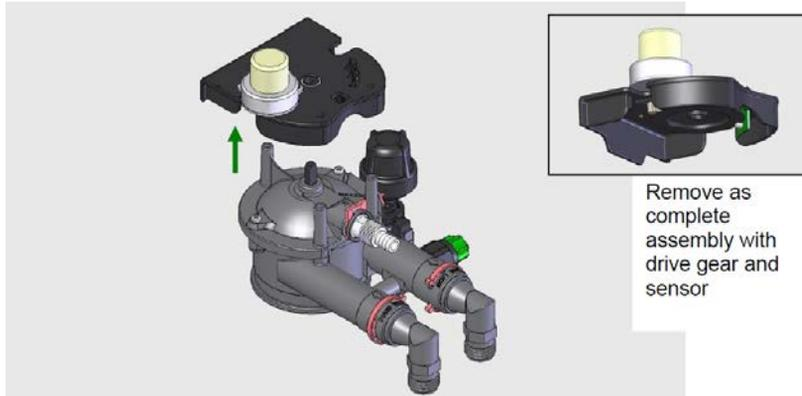
NOTE: It is now preferable to remove the opposite end of the sensor cable from the valve body so that the motor plate can be completely removed
