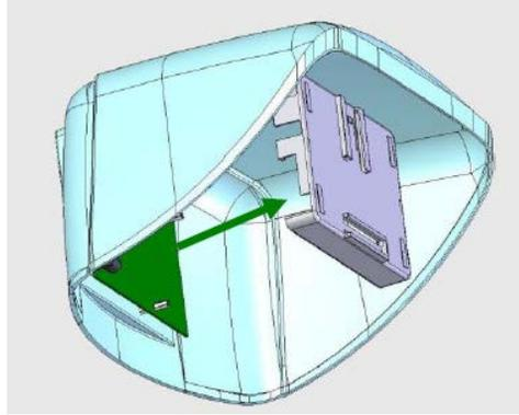
3.6. Disconnect the ribbon cables from the rear of the PCB (and any other connections such as the chlorination device if fitted). All cables are attached using discreet pin sockets and can be removed by simply pulling the white connector housing sideways off the pins attached to the PCB
