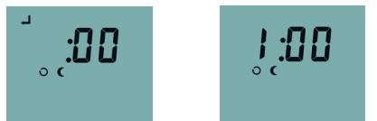
Pressing the [SET] key once enters the recharge time and moves the display into service mode.
