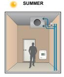
In 4-pipe installations, there are two separate water systems for heating and cooling with separate valves. The controller uses two outputs for control of heating and cooling in sequence with two thermal actuators.
