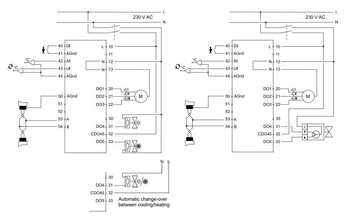
Wiring diagram for thermal actuator
