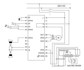
Wiring diagram with electric heater
