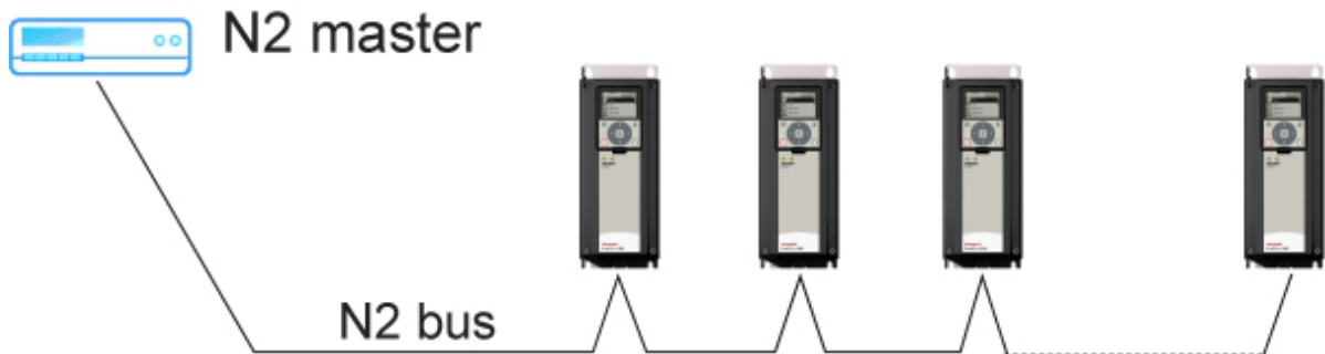
Figure 4. Principal example diagram of Metasys N2
